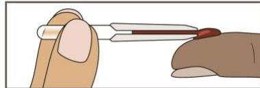
**CAUTION!** Filling is automatic: Never squeeze the tube while sampling. Don't squeeze the bulb; MICROSAFE® fills by capillary action.
